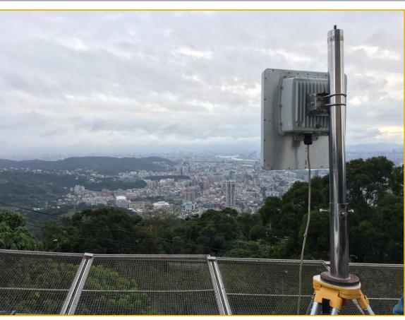
BS setup: HYC-N1051C-53 with 26dBi MIMO panel embedded
